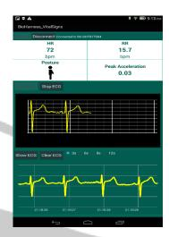
This application confirms the usefulness of the Zephyr Bioharness sensor in a hospital environment by providing remote monitoring of patient vital parameters. The application is set and tested in General Hospital in Celje, Slovenia.
